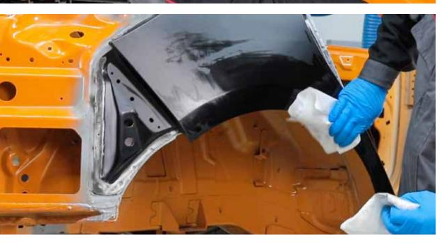
► Tool excess adhesive squeeze-out from repair area prior to curing to seal the repair
