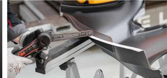
▶ Remove Ecoat from replacement panel mating flange areas using Scotch-Brite™ Belt
