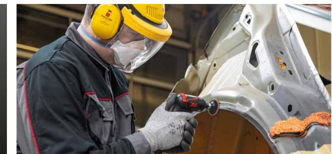
► Remove remaining material and contminants from host panel. Prep remaining mating flanges on host panel with a Scotch-Brite™ Belt or Disc
