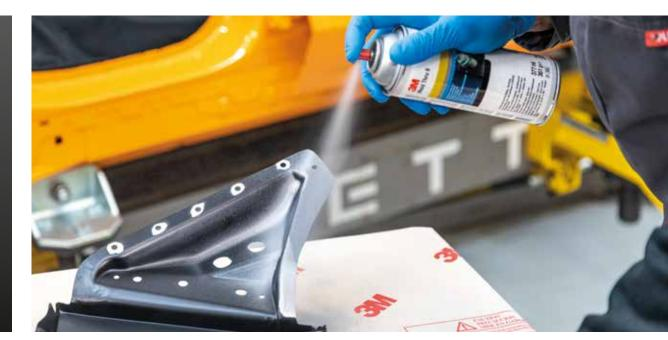
Apply weld-thru primer to all areas on host panel and replacement panel requiring welding operations, exept the areas for bonding
