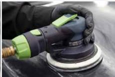
To reduce compounding time, refine the scratches left after the first step using the following 3M abrasives.
