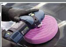
To remove the final sand scratches from the Micro Scratch Refinement step and bring up a high gloss finish, use 1-Step Finishing Material and Pads:
