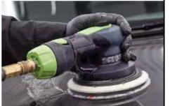
For the best results and the ultimate finish, further refine the 3000 scratches using the following 3M abrasive:
