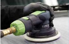
To remove dirt nibs and level excess surface texture over large or small areas use one of the following fine grade 3M abrasives:.
