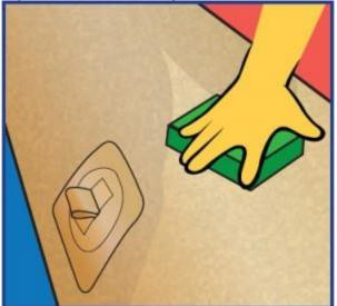
**4 CLEANING** The inflatable tubes must be cleaned of dirt, oxidation & grease by using Polymarine
