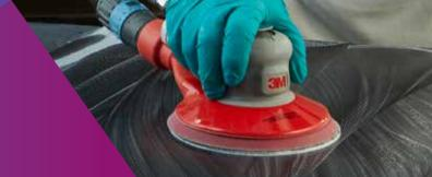
Paint imperfections can be removed using a 3M<sup>™</sup> 260L Micro Finishing Disc with an interface pad on a sander. For smaller areas, choose the appropriate abrasive grade and size, with the corresponding block from the 3M<sup>™</sup> Paint Defect Removal System.
