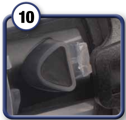
10 Inspect atomizing head for damage or wear which could result in fluid leaks or poor performance.
