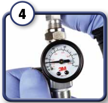
4 Set air pressure at 20 psi at full trigger (air and fluid flowing).
