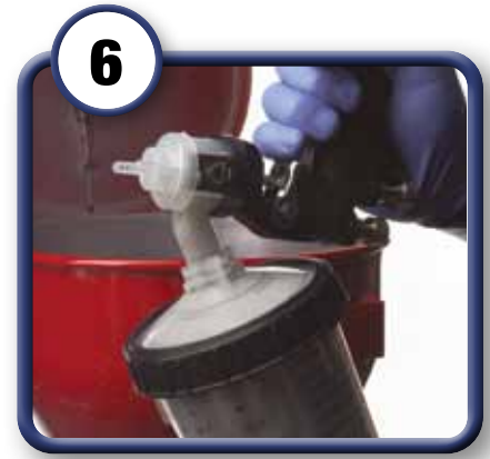
6 When you are finished using the system remove the air line and 3M™ PPS™ Cup.
