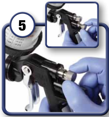
5 Adjust fan and fluid flow to achieve the desired size and wetness of the pattern. NOTE: when closing the fan adjustment completely it may be necessary to re-adjust the air flow control valve.
